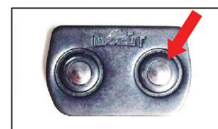
12) The picture on the right shows a repaired chain section.
