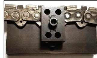
8) Install the Riveting Bit into a drill press.
