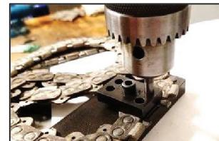
11) Check periodically until the rivet has formed over and is covering the chamfer on the Side Plate. Move to the second riveting bushing and repeat the process.
